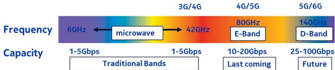
Evolution of WBH toward more capacity, includes the introduction of technique like the Cross polar canceller, alias XPIC, that allow to use the same channel two times, doubling the spectral efficiency and recently the Band and Carriers aggregation (BCA) [8], allowing to extend the reach of high-capacity link, exploiting the complementary performances of traditional bands link and E-Band link.
